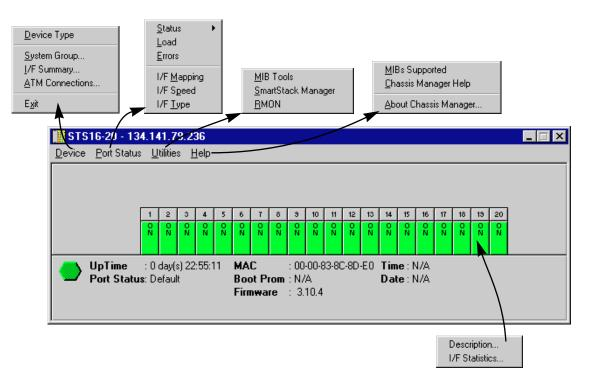
Figure 2-3. Sample Chassis View Menu Structure (STS16-20RM with an ATM SSIM)
